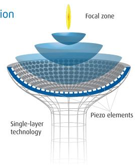
Piezo shockwave technology – **Direct Focusing**
