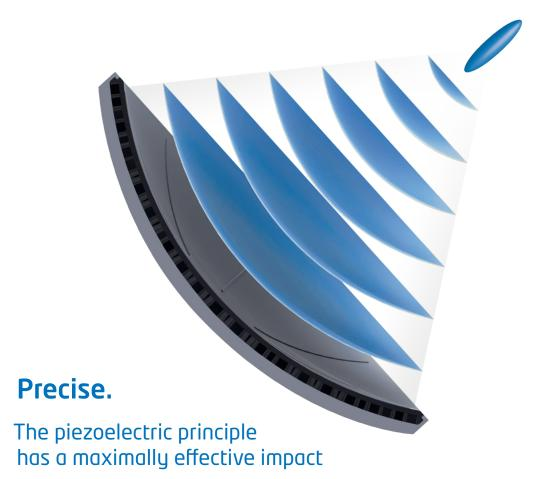
Piezo shockwave technology utilizes what is known as "direct focusing" and makes use of this principle in all of its therapy sources. This means that sound fields with the required output parameters for your respective treatment are generated directly – without "unnecessary" acoustic field deflections using reflectors or acoustic lenses and the potentially associated loss of performance.
